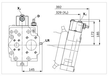
DR/DRG – Pressure controller/pressure controller remotely controlled
