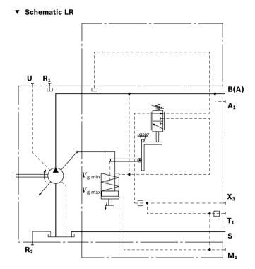
10 **A7VO Series 63** | Axial piston variable pump LR – Power controller without power override
