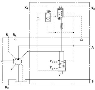
14 **A7VO Series 63** | Axial piston variable pump LA1 – Power controller with hydraulically proportional power override
