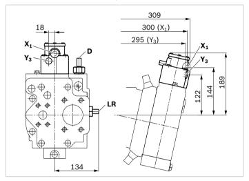
▼ LRDS – Power control with pressure cut-off and load sensing
