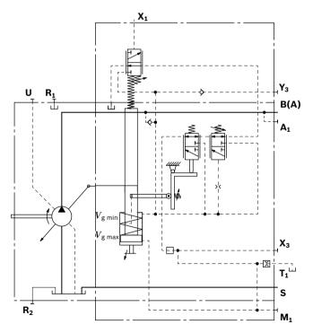
12 **A7VO Series 63** | Axial piston variable pump LR – Power controller without power override
