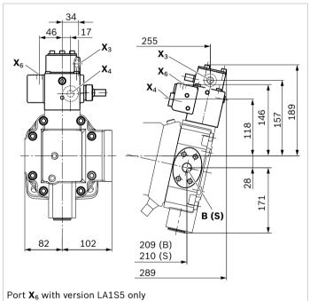
DR/DRG – Pressure controller/pressure controller remotely controlled
