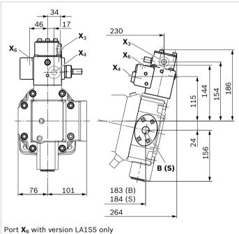
DR/DRG – Pressure controller/pressure controller remotely controlled
