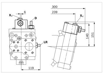
LA1S – Power control with load sensing,
