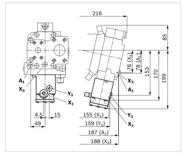
DR/DRG – Pressure controller/pressure controller remotely controlled
