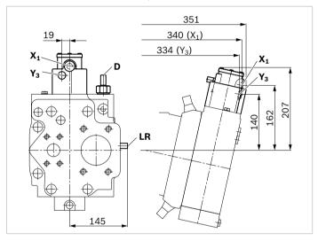
▼ LRDS – Power control with pressure cut-off and load sensing
