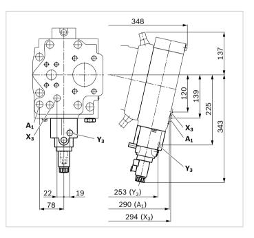
40 **A7VO Series 63** | Axial piston variable pump Connector for solenoids
