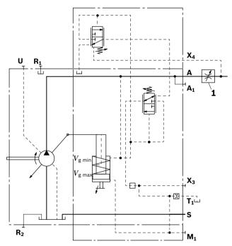
The measuring orifice (control block) (1) is not included in the scope of delivery.
