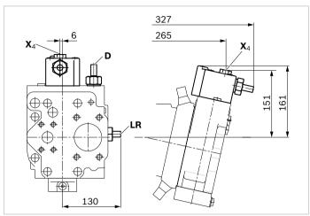
LA1S – Power control with load sensing,
