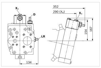
DR/DRG – Pressure controller/pressure controller remotely controlled
