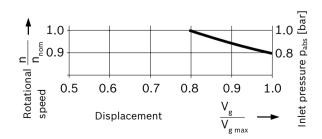
The inlet pressure is the static inlet pressure or the minimum dynamic pre-charge pressure value. Maximum permissible rotational speed  $n_{\text{nom}}$ , see page 7.
