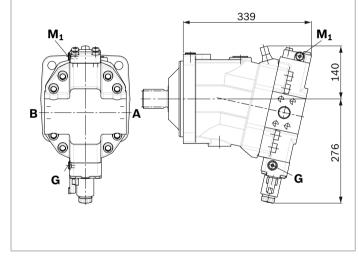
▼ DA0 - Automatic speed-related control, negative control, with hydraulic travel direction valve
