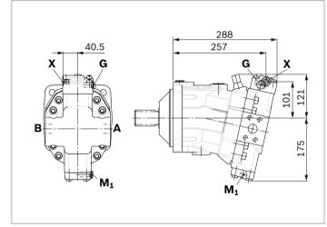
▼ **HZ7** – Hydraulic two-point control, negative control
