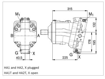
▼ HA1R1, HA2R2 – Automatic high-pressure-related control, positive control, with override, electric and travel direction valve, electric
