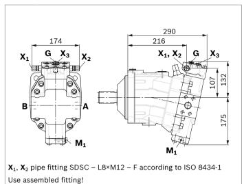
▼ DA1, DA2 - Automatic speed-related control, negative control, with electric travel direction valve and electric V<sub>g max</sub> circuit
