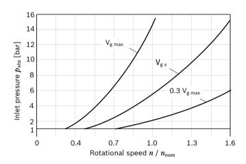
This diagram is valid only for the optimum viscosity range from  $v_{\text{opt}}$  = 36 to 16 mm<sup>2</sup>/s.
