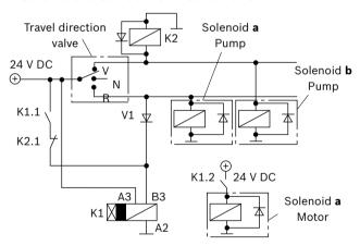
The diodes and relays shown are not included in the scope of delivery of the motor.
