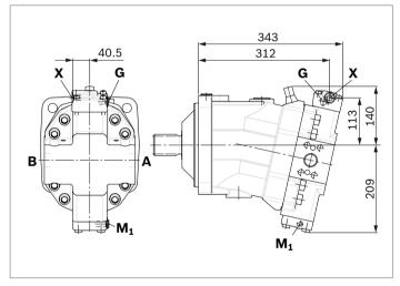
▼ HZ5 – Hydraulic two-point control, negative control
