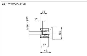
Involute spline acc. to ANSI B92.1a, 30° pressure angle, flat root, side fit, tolerance class 5
