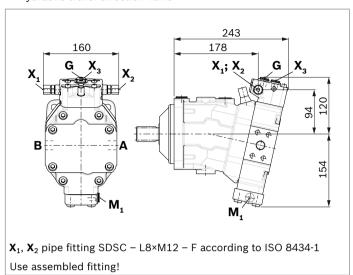
▼ DA1, DA2 - Automatic speed-related control, negative control, with electric travel direction valve and electric V<sub>g max</sub> circuit
