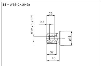
Involute spline acc. to ANSI B92.1a, 30° pressure angle, flat root, side fit, tolerance class 5
