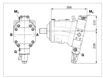
▼ DA0 - Automatic speed-related control, negative control, with hydraulic travel direction valve
