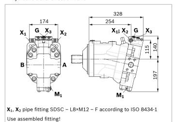
▼ DA1, DA2 - Automatic speed-related control, negative control, with electric travel direction valve and electric V<sub>g max</sub> circuit
